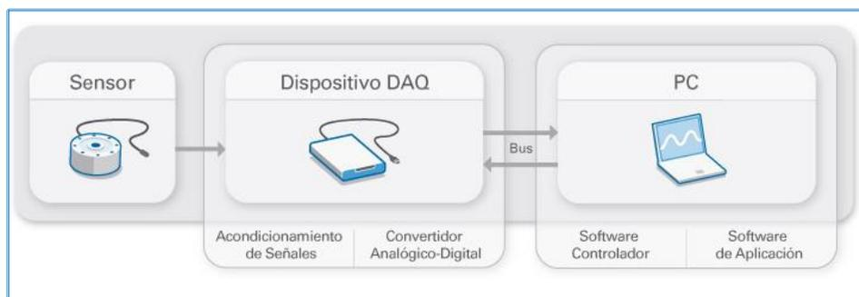
Figura 3.3. Partes de un sistema DAQ (National Instruments, 2018). Recuperado de: <https://www.ni.com/data-acquisition/what-is/esa/>
